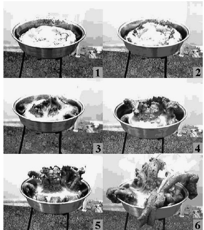
Fig. 2. Self-propagating combustion stages of the citrate–nitrate gel containing cationic surfactant.
